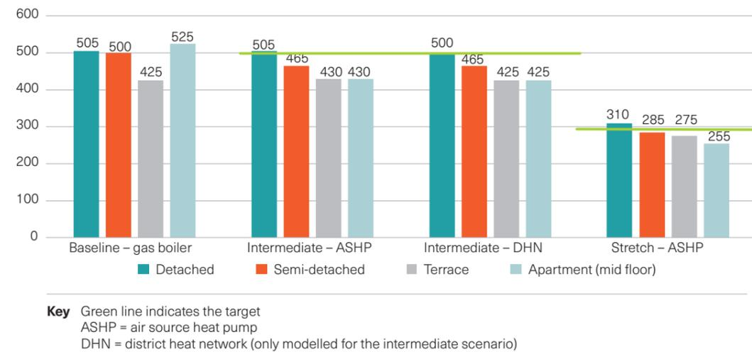
**Figure 5:** Embodied carbon results (modules A to C, excluding B6 & B7; kgCO<sub>2</sub>e/m<sup>2</sup>)
