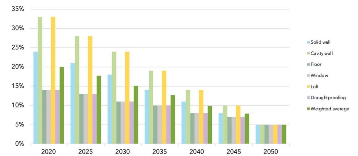
Figure 9: Performance gap factors for retrofit measures in existing homes
