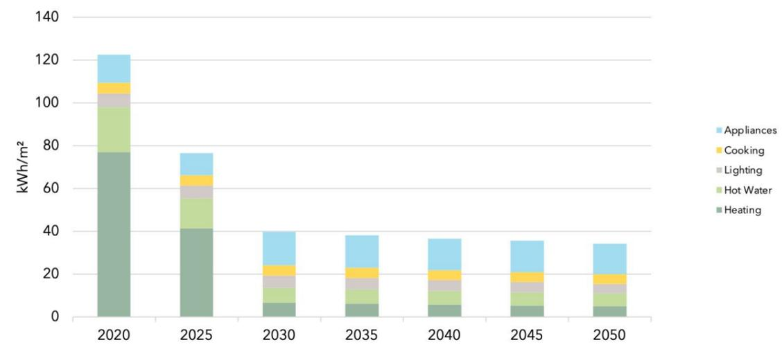
**Figure 16:** Resultant new dwelling energy use intensity (kWh/m²/yr)
