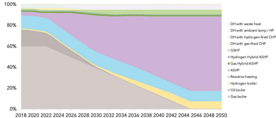
Figure 20: Non-Domestic Existing Building Heating Technology Mix
